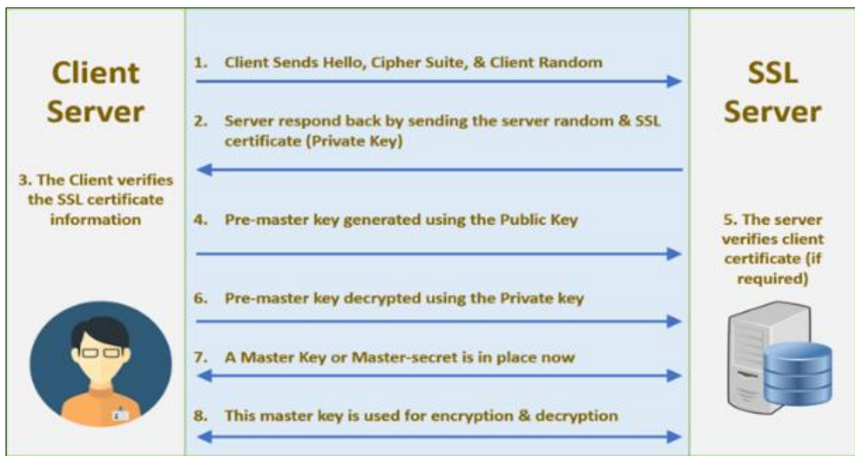
Figure 3 SSL Handshake process
