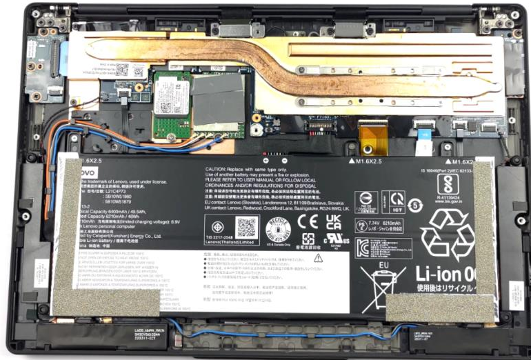
Figure 13 X13s with no CPU cooler
