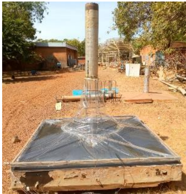
Figure 1 Photo of the prototype of the solar chimney
