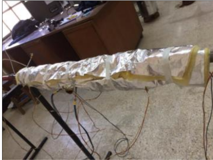
Figure 2 Test section fitted with insulation
