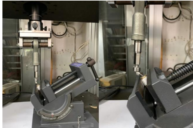
Figure 3 The compressive strength testing process on Ti-6Al-4V implants using the Hung Ta Type HT-9501 universal testing machine
