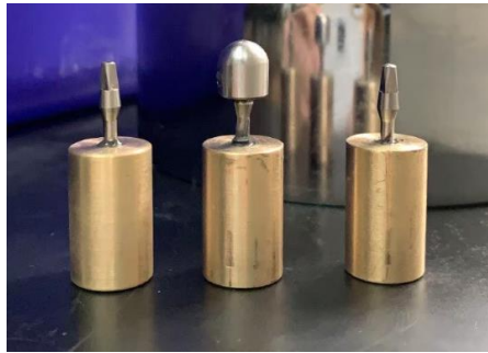
Figure 1 The assembled implant with brass rod and hemisphere before undergoing further testing
