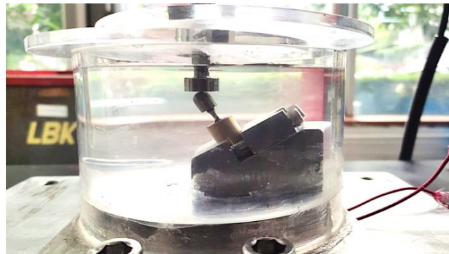
Figure 2 The immersion process with artificial saliva at pH 6.5 and dynamic treatment following ISO 14801 standards with a total of 2 million load cycles
