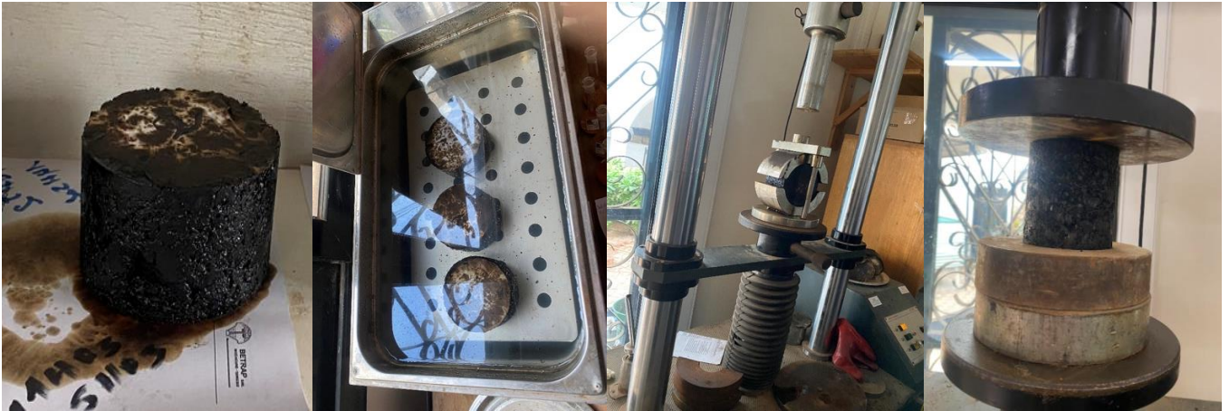
Figure 3 Marshall test molded samples and compression machines
