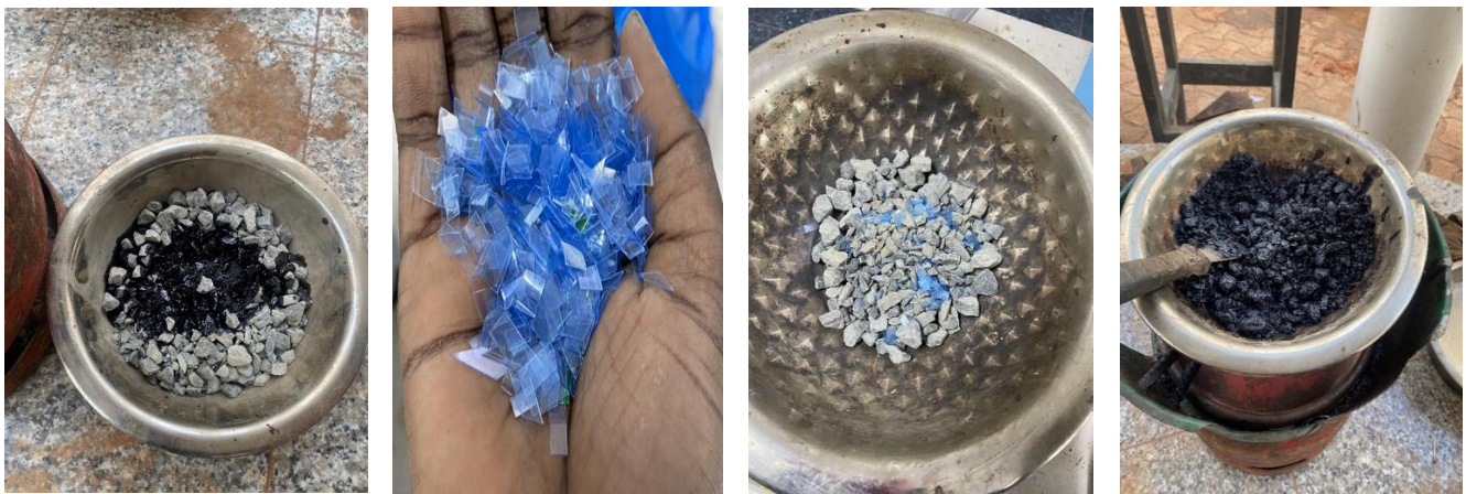
Figure 2 Preparation and addition of plastic waste in the aggregates before heating
