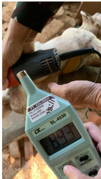
Figure 4 Sound Level Meter Measurement Results on a Hand Grinding Machine
