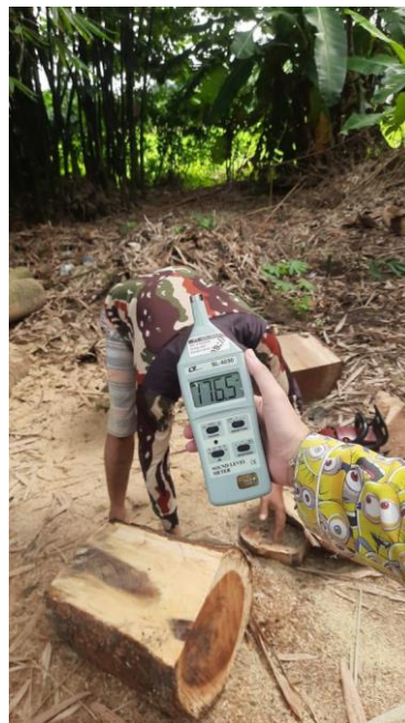
Figure 2 Sound Level Meter Measurement Results on the Senso Saw Machine
