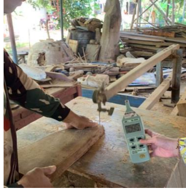
Figure 3 Sound Level Meter Measurement Results on the Bobok machine
