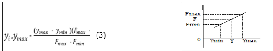
Figure 7 Determining the y_i deflection by linear interpolation
