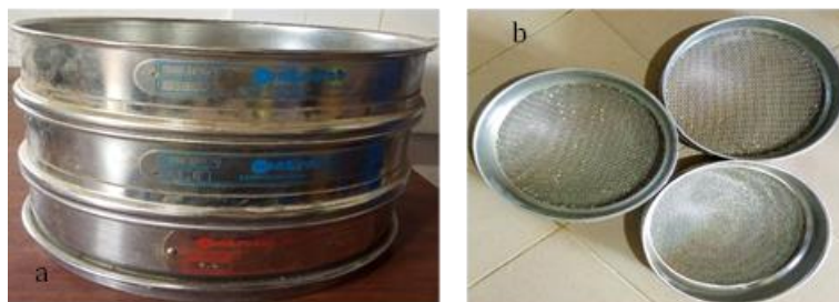
Figure 2 Sieves: a) side view of the different sieves; b) top and bottom view of the sieves
