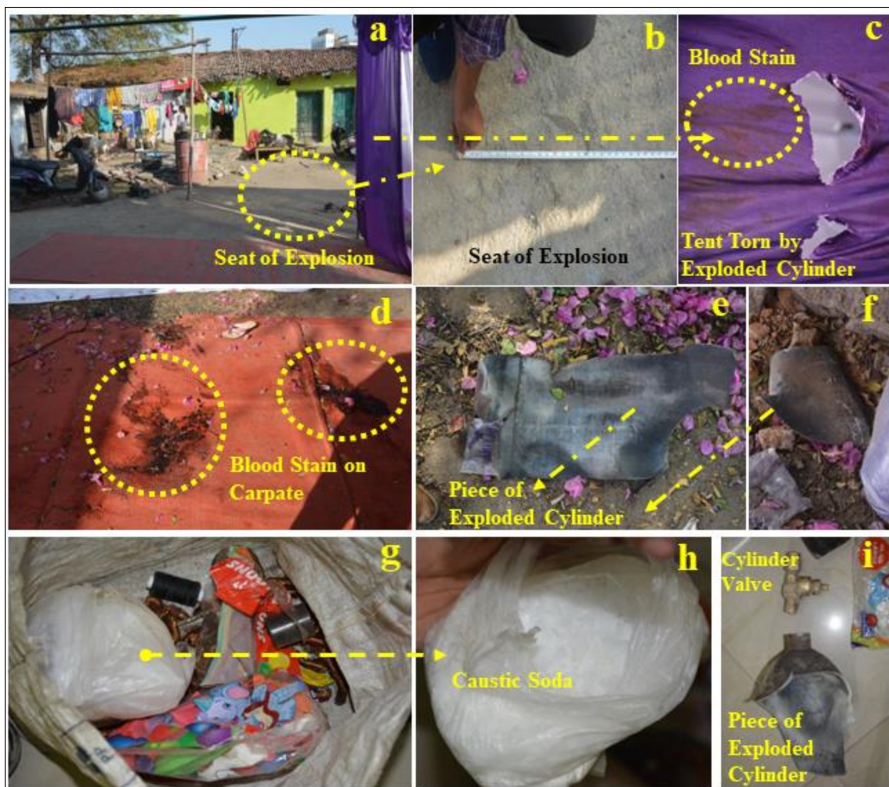
Figure 1 (a) Explosion Site (b) Seat of Explosion (c) Torn tent by exploded cylinder parts with blood stain (d) carpets with blood stains of injured (e and f) Pieces of exploded cylinder (g) recovered material from the site which contain caustic soda, balloons etc. (h) Caustic soda recovered from the explosion site (i) cylinder valve and exploded cylinder piece.
