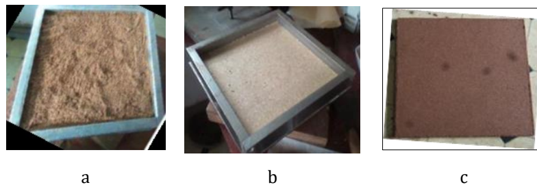
Figure 2 Thermal pressing steps: mixture in the mould (a), particleboard pressed (b), unmoulded particleboard (c)
