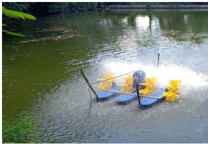
Figure 1 04 Paddle wheel aerator
