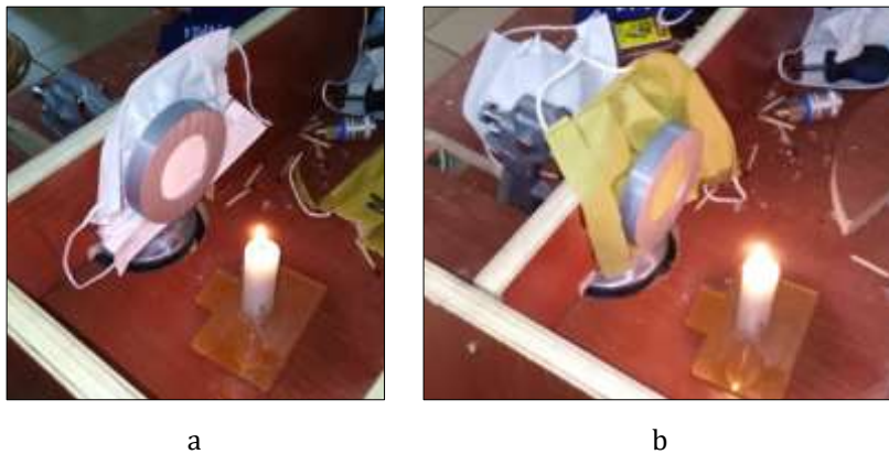
Figure 3 Mask candle flame test; a. Validation with surgical mask ; b. Local mask testing
