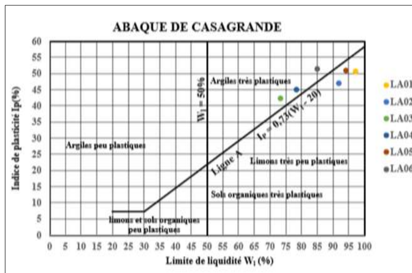
Figure 2 Liquid limit and plasticity index of the soils studied plotted on the Casagrande plasticity diagram
