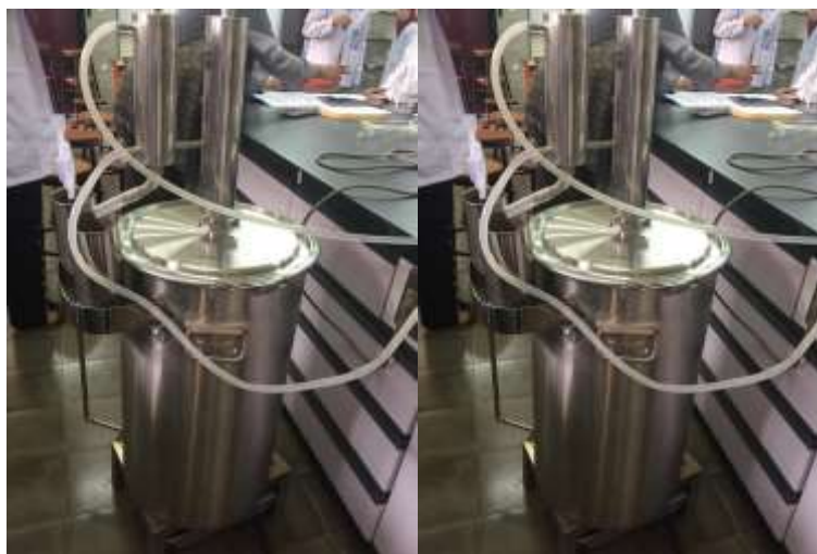
Figure 1 Distilled boilers for steam-hydro distillation
