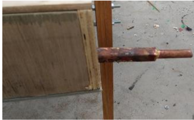
Figure 5 End Connection of Solar Water Heater
