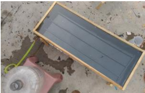
Figure 8 Square Tube Solar Water Heater Experimental Setup
