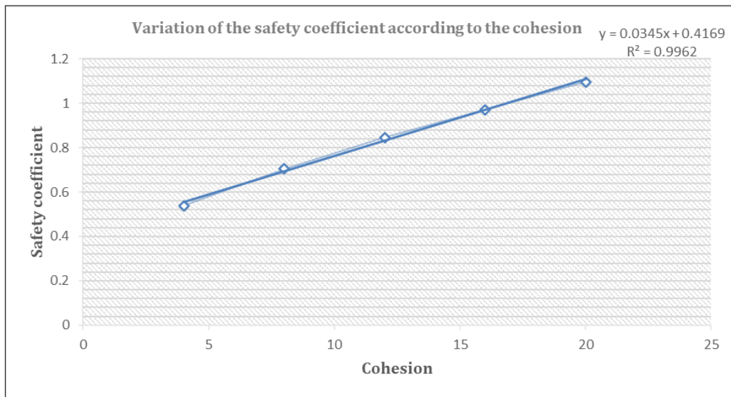
Figure 12 Variation of the safety coefficient as a function of cohesion by the numerical method
