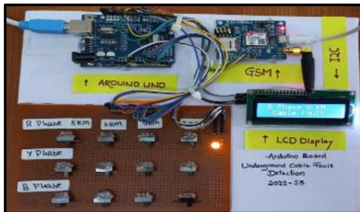
Figure 5 Cable Fault Detected at B-Phase ( 8Km Distance)
