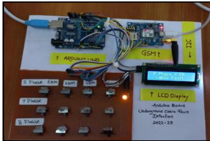
Figure 7 Cable Fault Detected at R-Phase ( 2Km Distance)
