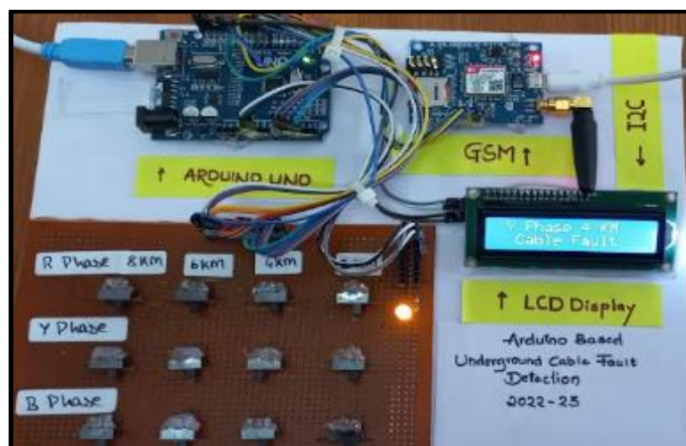
Figure 6 Cable Fault Detected at Y-Phase ( 4Km Distance)
