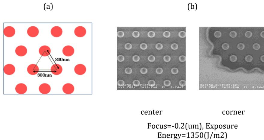
**Figure 1** (a) 400nm in diameter and 800nm in pitch arranged triangular lattice. (b) The SEM photo at center and corner of the exposure field
