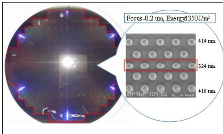
**Figure 3** CD-error to the edge of exposure field
