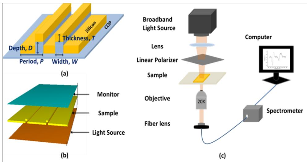
**Figure 1** (a) Schematic of a dual-layer silicon nanoslit array. (b) 3D simulation model of the silicon nanoslit array. (c) Measurement setup
