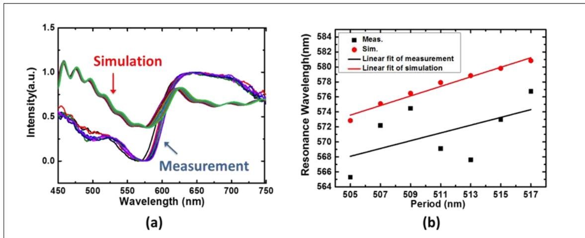
**Figure 2** (a) Simulated and measured transmission spectra of silicon nanoslit array with different slit periods. (b) Simulated and measured resonance deep wavelength of silicon nanoslit array with different slit periods
