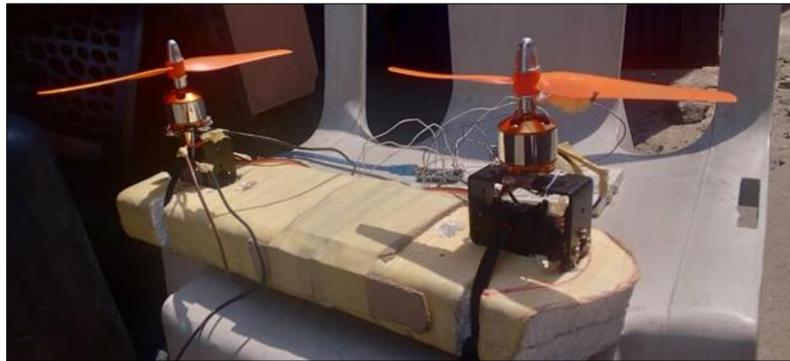
**Figure 7** The assembled Drone
