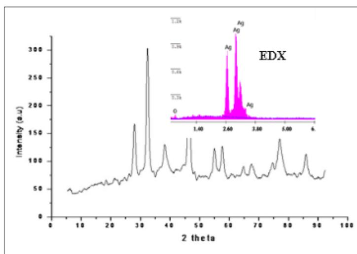
**Figure 4** XRD spectrum of synthesized and stabilized AgNPs at peak 29.50° and 32.50° depict crystalline nature with average grain size of 25.5 nm. Inset is EDX spectrum showing Ag alone.
