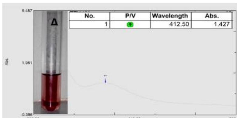
**Figure 2** Confirmation of biogenic AgNPs synthesis by UV-Vis spectrum using free and conjugated amines at absorbance wavelength peak at 412.5 nm, inset (A) shows brown colour indicating formation of AgNPs
