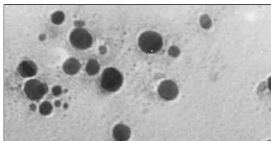
**Figure 3** TEM analyses of AgNPs synthesized and stabilized by amines indicating spherical shaped measuring 8-50nm with an average of 25.5 nm.
