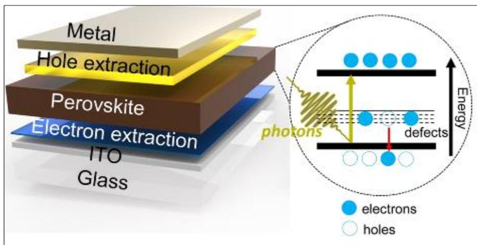
**Figure 2** The charge-transfer process and energy levels of OIP solar cells [24]
