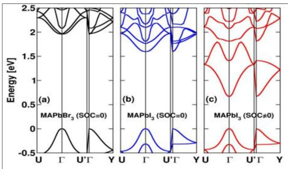
**Figure 3** The band structures of OIP with and without Spin-orbiting coupling (SOP)
