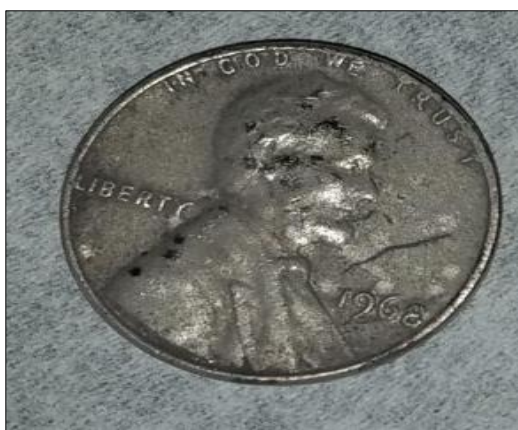
Figure 6 Electroless Nickel coated Penny
