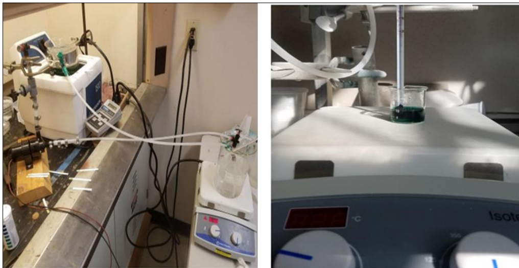
Figure 2 Electroless nickel plating setup with ultrasonic bath and water pump
