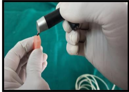
Figure 3 sandblasting with alumina particles
