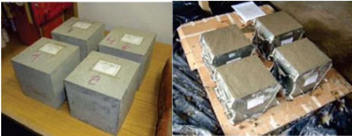
Figure 3 Concrete cubes after de-moulding, in wrapped state
