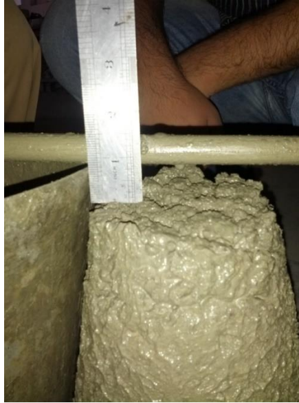
Figure 4 Slump Value Test; Slump Value coming out to be more than 1”
