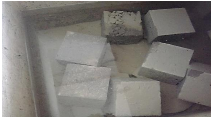
Figure 2 Concrete cubes being cured in Ponding Tank
