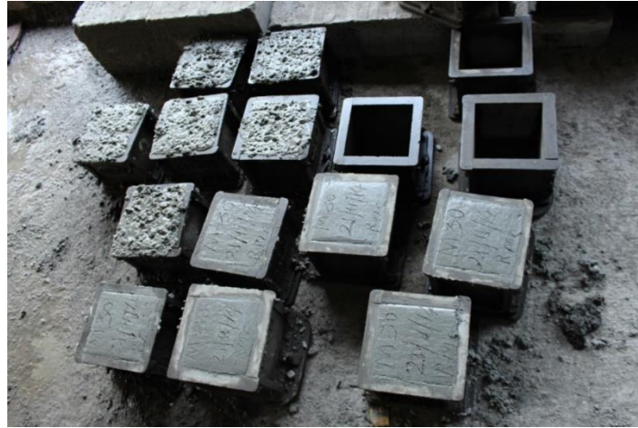
Figure 1 Concrete cubes being placed in moulds
