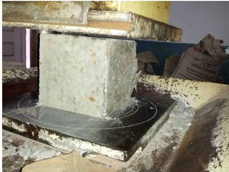
Figure 6 Concrete being tested under Compression Testing Machine
