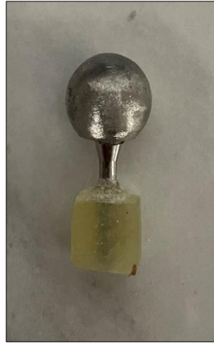
Figure 2 Ti-6Al-4V implant with implant holder made of ARALDITE® Standard Setting Epoxy Glue and specimen head made of VERABOND® Nickel Chromium
