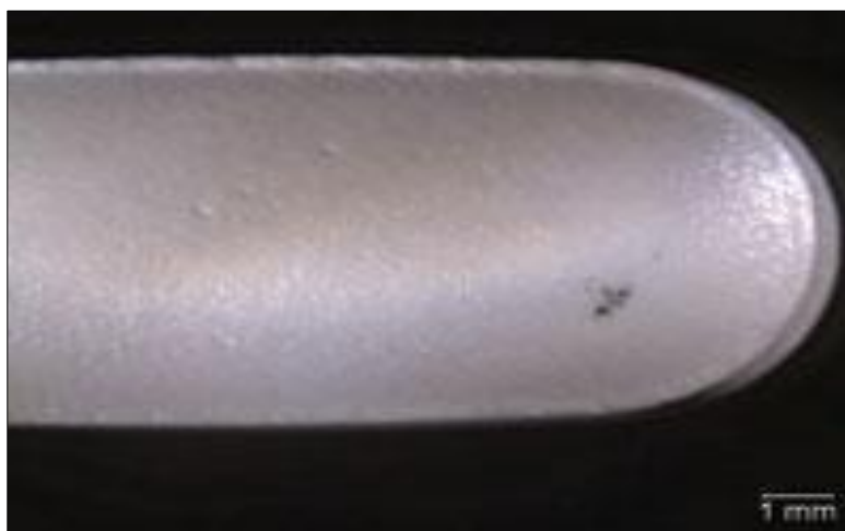
Figure 1 Metal particle in a compressed tablet [5]
