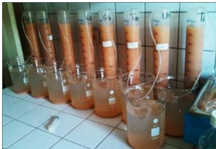
Figure 2 Communicating vessel system for the extraction of the fraction < 2 \mu\text{m}
