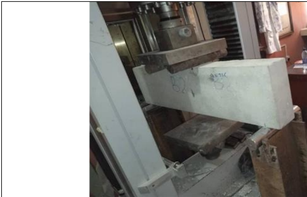
Figure 3 Typical set-up of universal testing machine
