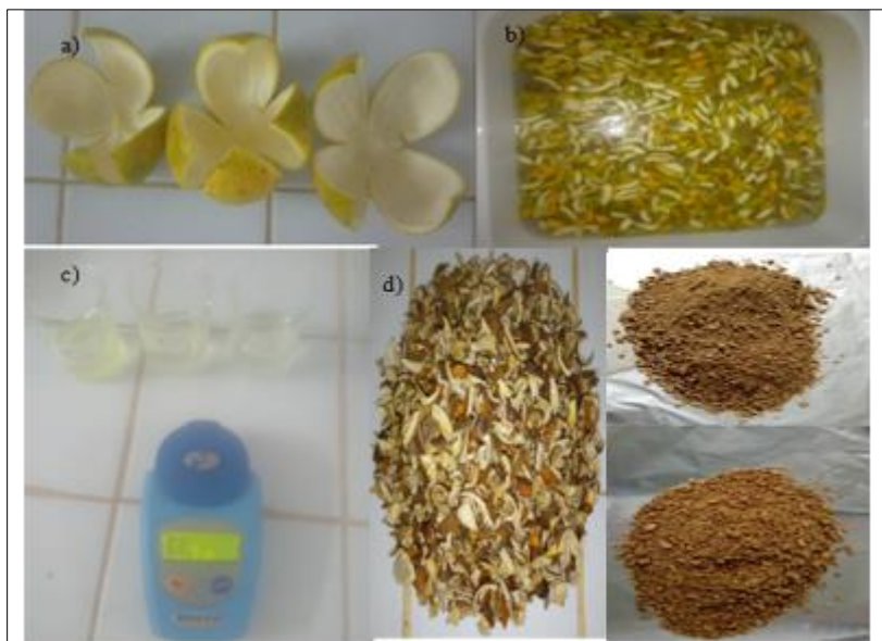
Figure 2 Isolation and grinding of orange peels a) orange peel; b) cut bark; c) determination of the Brix degree; d) dried and ground bark
