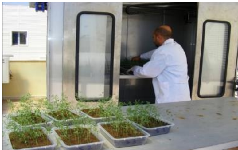
Figure 3 Full automated cabinet sprayer used to apply imazamox to lentil cultivars included in the study
