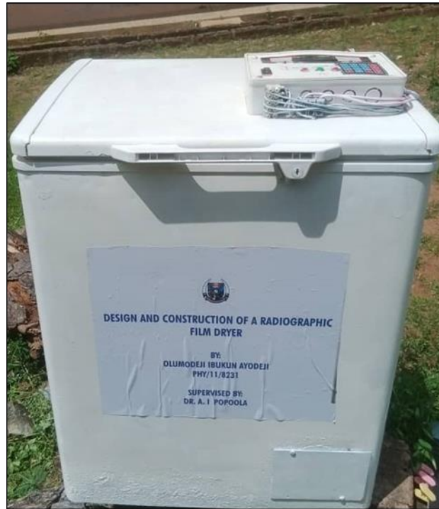
Figure 6 The constructed Radiographic Film Dryer
