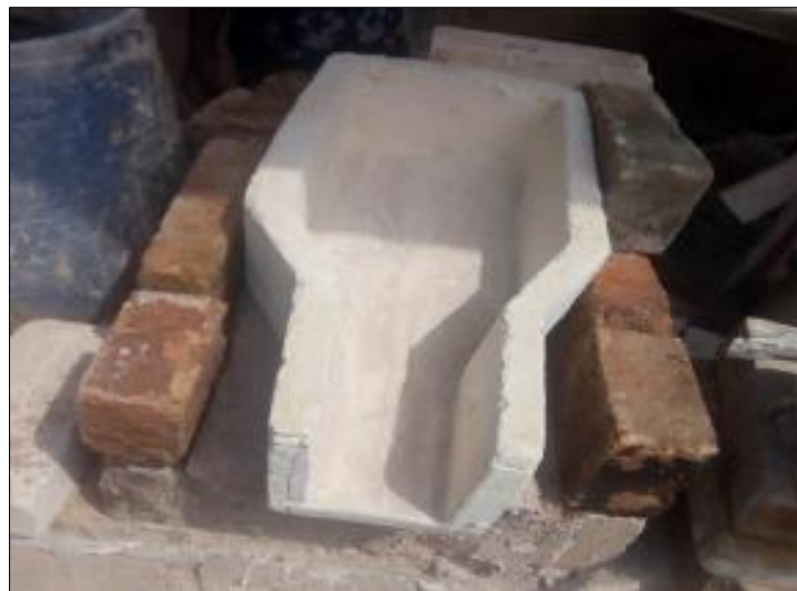
Figure 6 Fired lining in Place within the Furnace Wall
