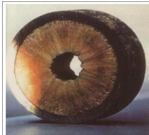
Figure 8 Cross-section of a pipe with deposited wax [3, 10, 33, 35, 37]
