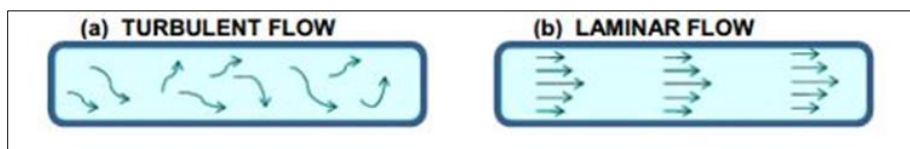
Figure 3 Orientation of fluid molecules during (a) Turbulent flow and (b) Laminar flow [27]
