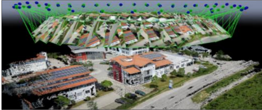
Figure 6 Aero triangulated images and generated 3D point cloud using Pix4D App
