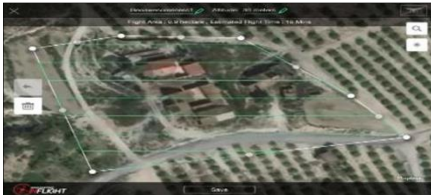
Figure 7 The autopilot follows the routes identified after mapping the area on the map
