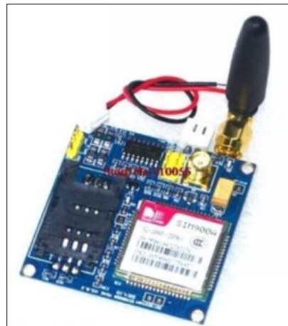
Figure 6 GSM Module used for the construction of GSM Based home security alert using PIR Sensor
