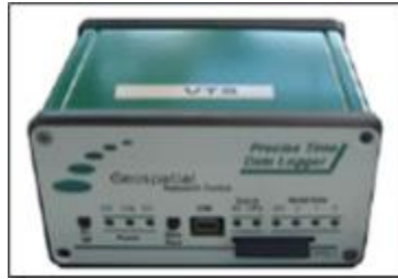
Figure 15 DLSU: data logger and synchronizer sensor
