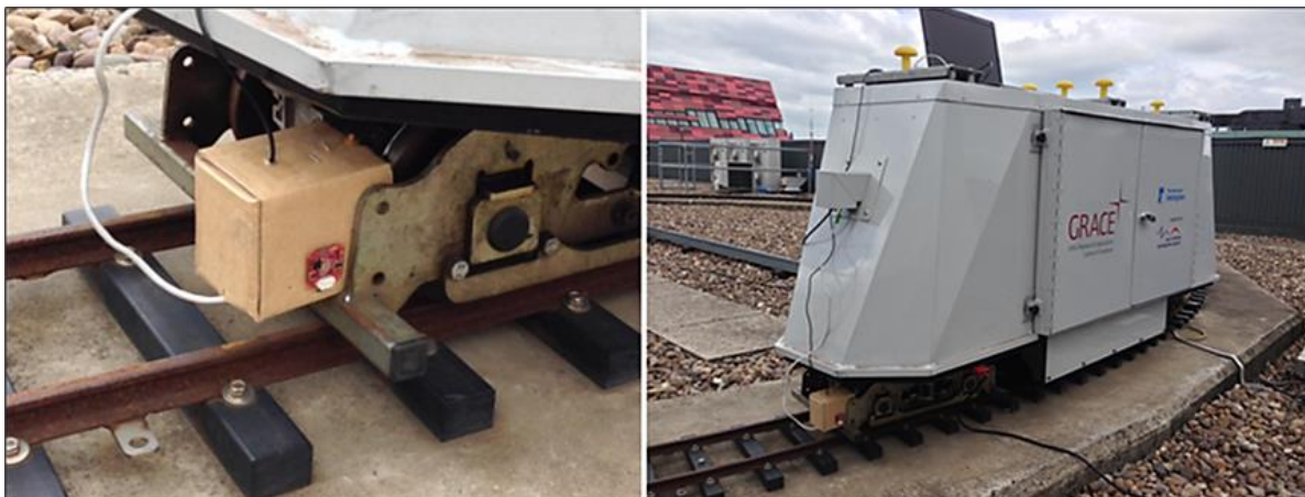
Figure 21 GNSS/INS testing train of NGI with MSL, SPL, IMU, camera, and GPS
