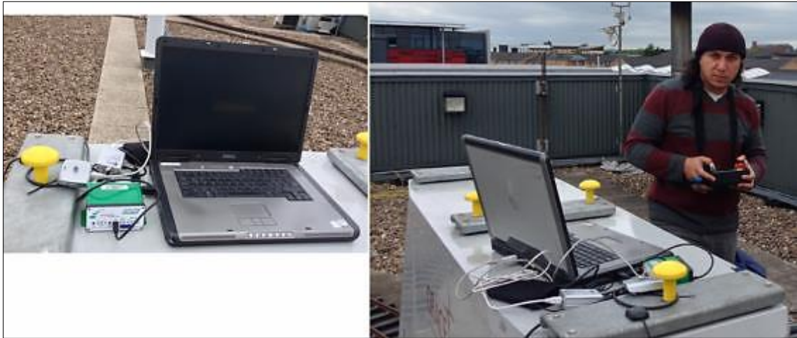
Figure 22 DLSU, u-blox GPS receiver, & DPU
