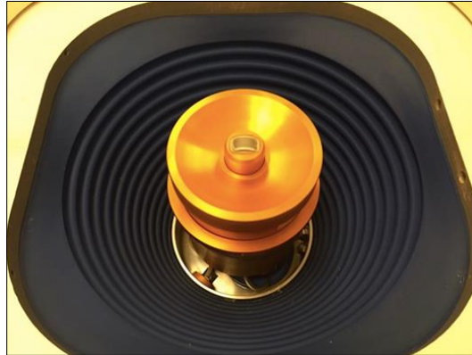
Figure 2 Real-time diagnostic ultrasound scanner integrated in the centre of the therapeutic ultrasound transducer
