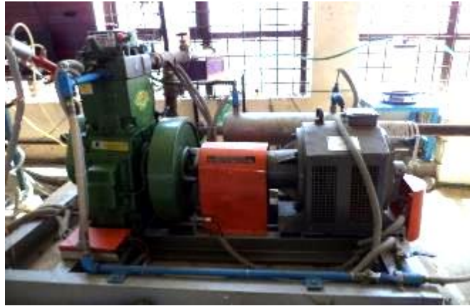
Figure 6 Single cylinder 4 stroke diesel engine
