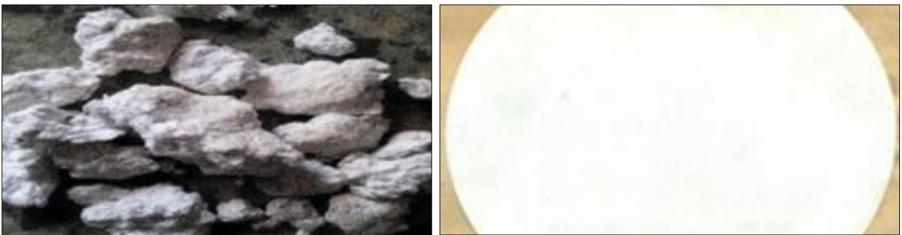
Figure 16 EFB Pulp Samples from MEA Process Bleached to 12.7 Kappa Number and Pulp sheets
