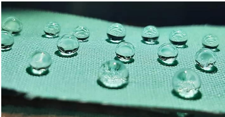
Figure 8 CCD image of different water droplet on the SiNPs coated cotton sample after PFOTS, showing the beautiful superhydrophobic view.
