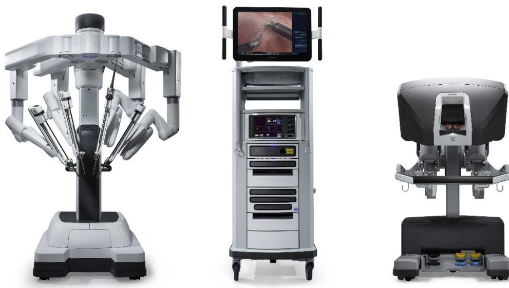
Figure 2 Da Vinci Image, Xi, Trio of System Components. Image of complete da Vinci Xi System including the patient side cart, vision cart and the surgeon console.
