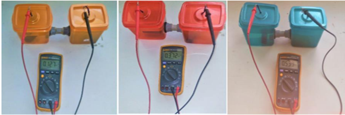
Figure 1 Voltage measurement for glucose optimization using digital multimeter
