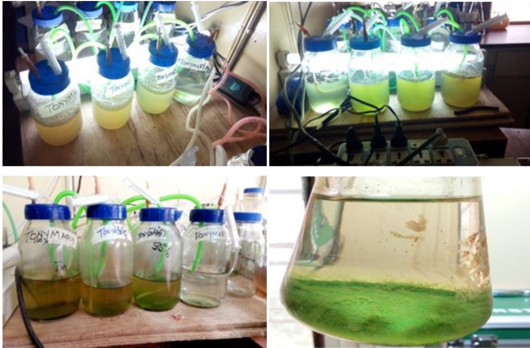
Figure 3 Showing from up-left; days 2, 5, 10 and 15 of microalgae cultivation. At day 15, microalgae have taken up all the nutrients especially the Total phosphorus content and soluble solids present in the sewage effluent broth.
