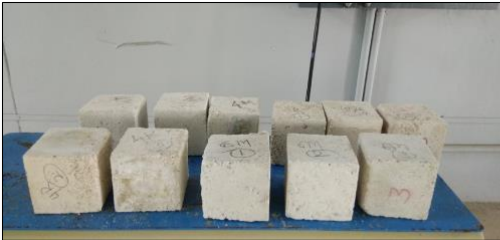
Figure 15 Mortar cubes after acid attack
