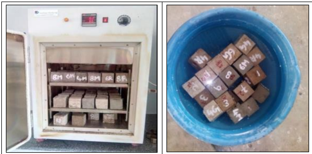
Figure 10 Set up for water absorption test
