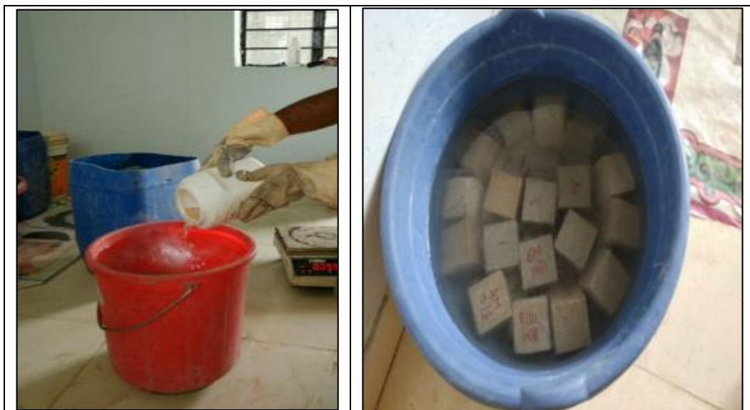
Figure 14 Set up of acid resistivity test
