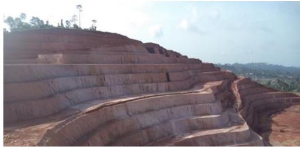
Figure 2 A quarry showing staged ore extraction (saprolite ramps)
